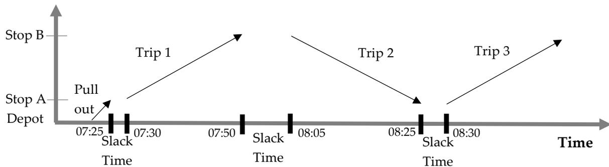
Figure 1. Slack time diagram.
