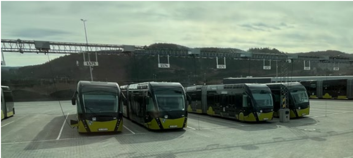
Figure 3. Buses charging at the depot in Trondheim
